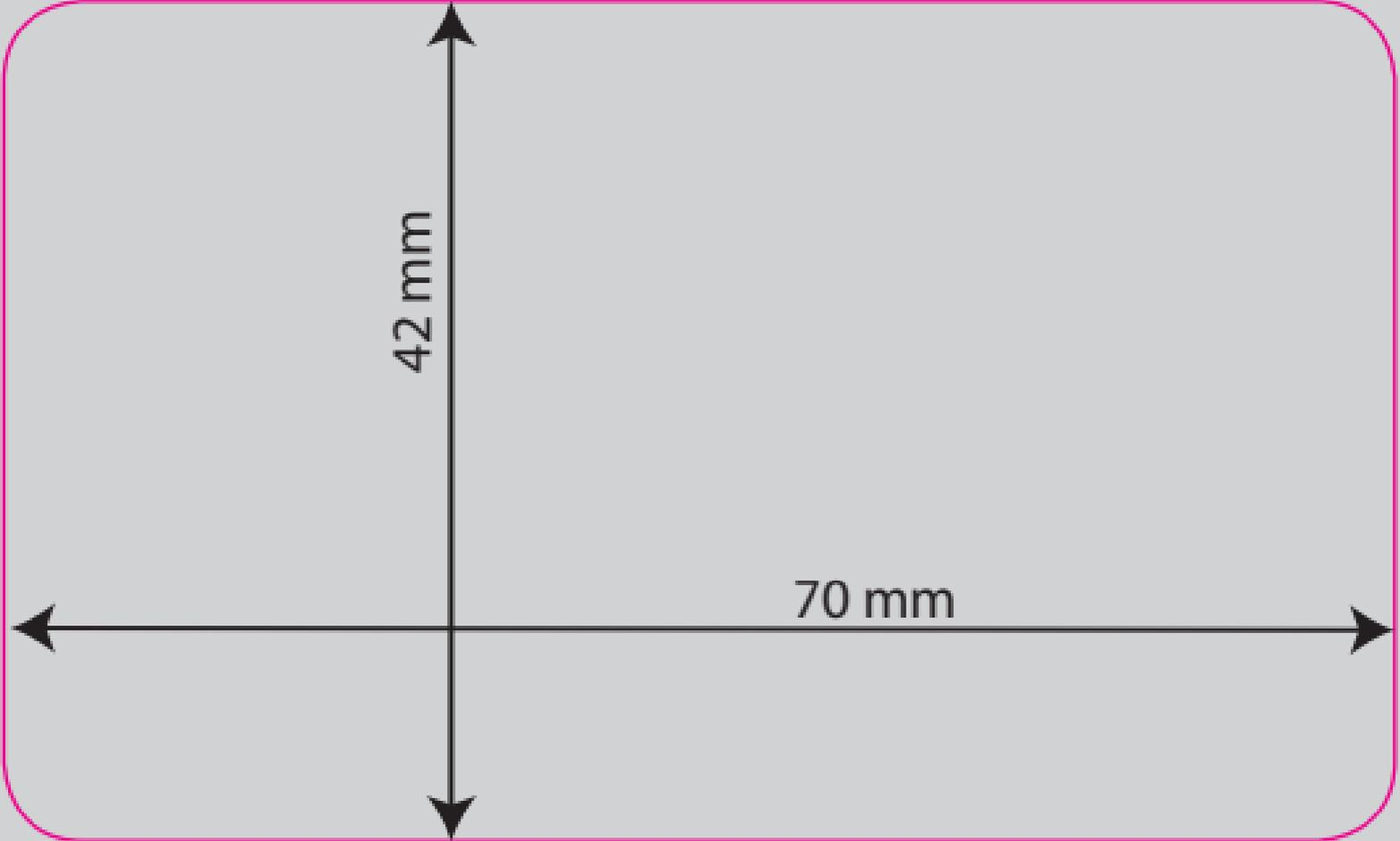
A diagram of a rectangular plate with rounded corners, outlined in pink. A vertical dimension line with arrows at both ends is labeled "42 mm". A horizontal dimension line with arrows at both ends is labeled "70 mm".
